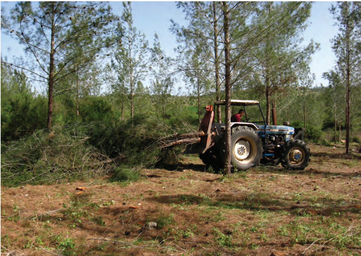
Removing cut trees by skidding during thinning. Aleppo pine forest in Adulam Park in the Judean Lowlands.
