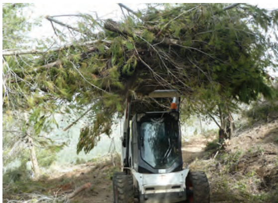
Removal of cut woody material with a small articulated loader from a coniferous forest after thinning. Aminadav Forest, Judean Mountains.
